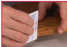
10. Remove the excess with a plastic card or putty knife.
